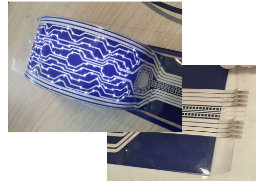
Overmolded flat interconnect (recycled PET)
