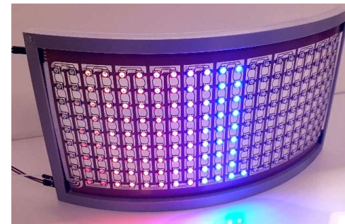
LEDs soldered onto printed Cu circuitry
